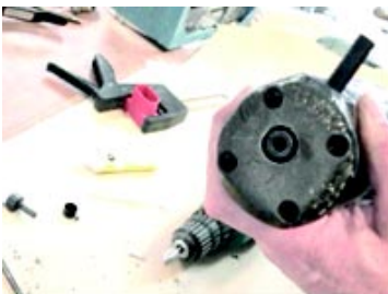
Insert guide pin up to its' second click. This creates glue guide for pin cap.
