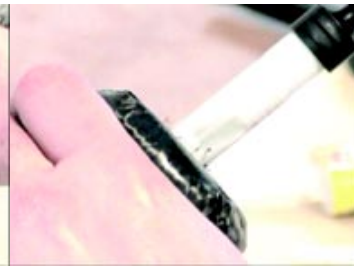
From end of socket use hole saw to drill hole to the bottom of the lock
